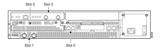
Slots in the Cisco 7140 series routers are numbered as shown in Figure 8-6. The fixed LAN interface is slot 0, the fixed WAN interfaces are slots 1 and 2, and the modular port adapter interface is slot 4. Slot 3 is not used. Slot 5 is the service adapter.
